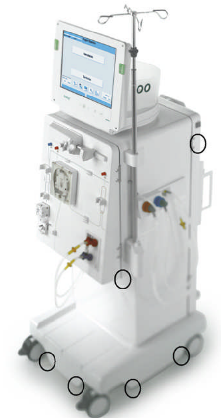
Fig. 3-2 Holding points for carrying the dialysis machine
